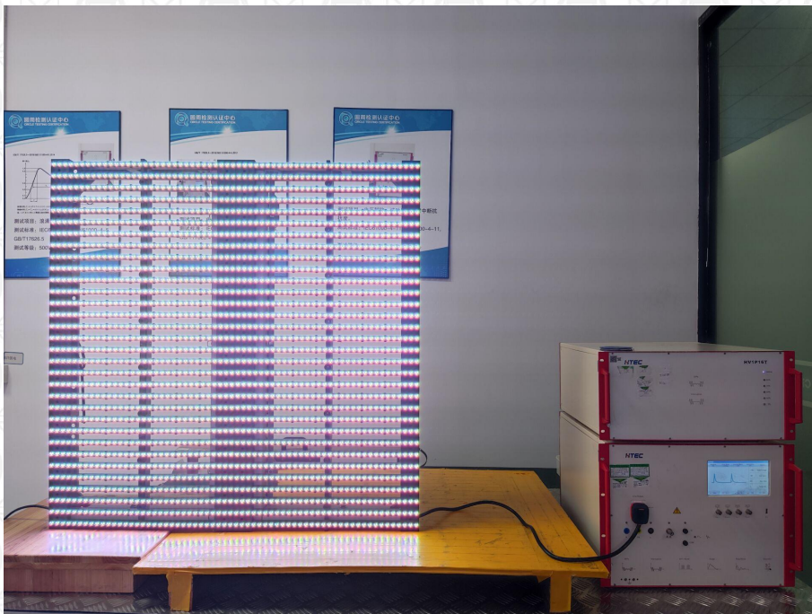
Figure 6: EFT/AC-DIP & Surge Test Setup
